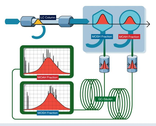
As described in the DIN EN 16995:2017-08 standard, volatile compounds are retained by solvent trapping applying partially concurrent eluent evaporation. High boiling compounds spread over the entire length of the flooded zone and are refocused using the retention gap technique. The dual channel GC/FID system enables simultaneous determination of the MOSH and MOAH fractions in 30 minutes.
