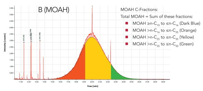
Unresolved complex mixtures (UCM) of MOSH (A) and MOAH (B) fractions extracted from an edible oil sample and integrated using the GERSTEL MOSH/MOAH Data Analysis software. The colored peak (signal) areas represent individual c-fractions (see tables). The total amounts are calculated as the sum of all c-fractions between  $n-C_{10}$  and  $n-C_{50}$ . The values are included in the final report.
